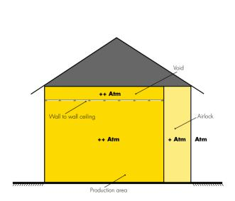
Ecophon Hygiene System is suitable as a sound-absorbing ceiling in constructions where there is equal pressure below and above the ceiling.
